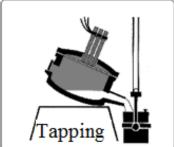
The EAF process is a form of secondary steelmaking. It is a batch process, meaning a specific amount of material is processed at a time, unlike the continuous nature of a blast furnace. The process flow is as follows:
